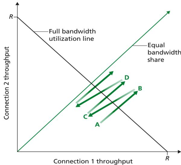
**Figure 3.53** ♦ Throughput realized by TCP connections 1 and 2
