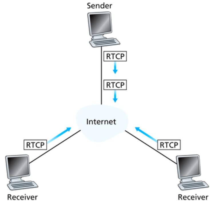
**Figure 7.13** ♦ Both senders and receivers send RTCP messages.
