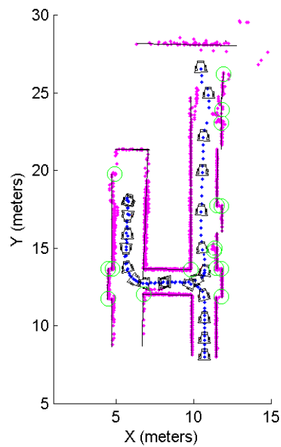
Figure 7: Map reconstruction of the facilities of the Instituto de Automatica . The magenta points are raw laser data; the solid black segments represent walls from the environment; green circles are corners and the blue dotted line is the path traveled by the mobile robot.
