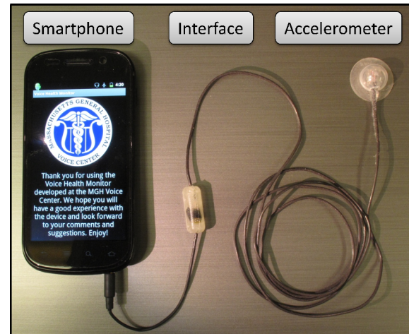
Figure 2: Ambulatory voice monitor currently under development that utilizes a smartphone as a data acquisition device, a similar accelerometer assembly for sensing neck-skin vibration, and an interface circuit to provide power to the accelerometer and impedance matching with the smartphone.
