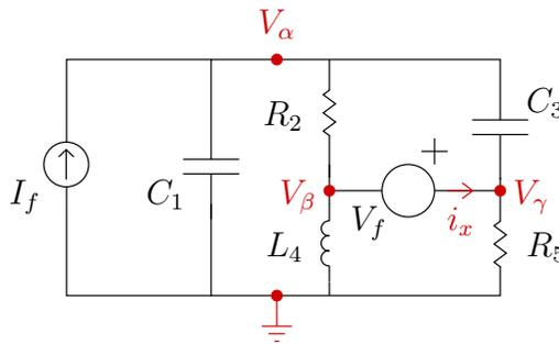
$$\begin{bmatrix} C_1D + \frac{1}{R_2} + C_3D & -\frac{1}{R_2} & -C_3D \\ -\frac{1}{R_2} & \frac{1}{R_2} + \frac{1}{L_4}D^{-1} & 0 \\ -C_3D & 0 & C_3D + \frac{1}{R_5} \end{bmatrix} \begin{bmatrix} V_\alpha(t) \\ V_\beta(t) \\ V_\gamma(t) \end{bmatrix} = \begin{bmatrix} I_f(t) \\ -i_x(t) \\ i_x(t) \end{bmatrix}$$
