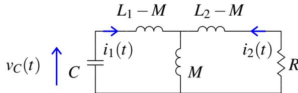
$$E_T = \frac{1}{2} C v_C^2(0) + \frac{1}{2} (L_1 - M) i_1^2(0) + \frac{1}{2} (L_2 - M) i_2^2(0) + \frac{1}{2} M (i_1(0) + i_2(0))^2$$
