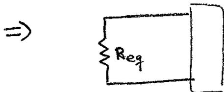
$$R_{eq} = R_1 \parallel \frac{1}{k} \parallel R_3 = \left( \frac{1}{R_1} + k + \frac{1}{R_3} \right)^{-1}$$
