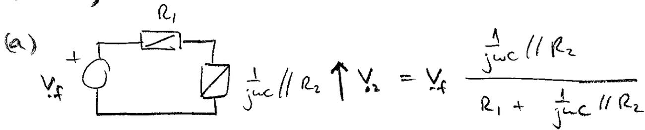
$$\frac{\frac{1}{j\omega C} \parallel R_2}{\frac{1}{j\omega C} + R_2} = \frac{R_2}{1 + j\omega C R_2}$$
