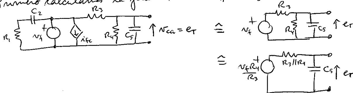
$$\Rightarrow e_T(t) = \frac{V_f R_4}{R_3} (1 - e^{-\frac{t}{\tau}}) \mu(t)$$
