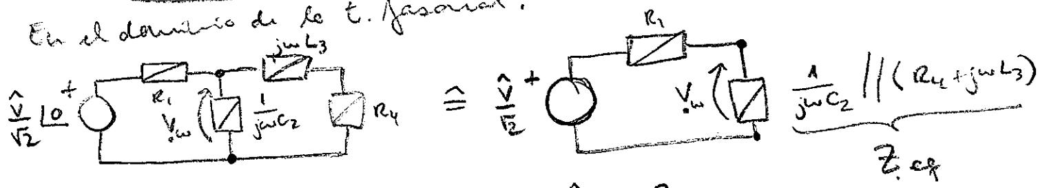
$$\Rightarrow V_\omega = \frac{\hat{V}}{\sqrt{2}} \frac{Z_{eq}}{Z_{eq} + R_1}$$
