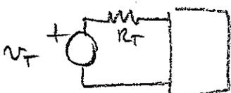
$$R_T = R_1 || R_2 || \left(-\frac{R_2}{k}\right)$$
