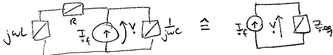
$$\text{en que } I_f = \frac{1}{j\omega} \text{ y } Z_{eq} = \frac{1}{jwC} \parallel (jwL + R) \\ = \frac{\frac{1}{jwC}(jwL + R)}{\frac{1}{jwC} + jwL + R} = \frac{jwL + R}{(1 - \omega^2 LC) + jwRC}$$
