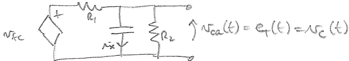
$$\frac{v_c}{R_1} + i_x + \frac{v_c}{R_2} = 0 \quad \left| \begin{array}{l} \left( \frac{1}{R_1} + \frac{1}{R_2} \right) v_c + \left( 1 - \frac{k}{R_1} \right) C \frac{dv_c}{dt} = 0 \end{array} \right.$$
