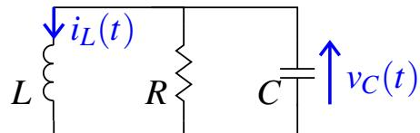
**Problema 7.3** Considere la red de la figura, donde  $R_1 = 1 \text{ [k\Omega]}$ ,  $R_2 = 2 \text{ [k\Omega]}$ ,  $C = 1 \text{ [\mu F]}$ ,  $L = 1 \text{ [H]}$ ,  $I_f = 3 \text{ [mA]}$ ,  $v_C(0) = 0 \text{ [V]}$  e  $i_L(0) = 0 \text{ [mA]}$
