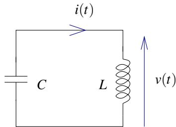
**Problema 7.2** Considere la red de la figura, donde  $R = 1 \text{ [k\Omega]}$ ,  $C = 1 \text{ [\mu F]}$ ,  $L = 1 \text{ [H]}$ ,  $v_C(0) = 1 \text{ [V]}$  e  $i_L(0) = 0 \text{ [mA]}$
