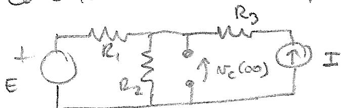
$$\text{Si } I=0 \Rightarrow [v_c(\infty)]_2 = \frac{R_2}{R_1 + R_2} E$$
