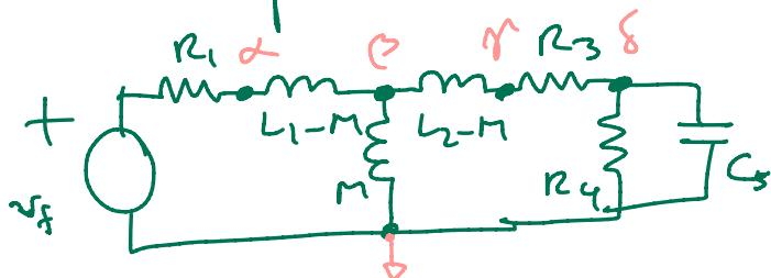
$$\alpha: \frac{v_\alpha - v_\beta}{R_1} + \frac{1}{L_1 - M} \int (v_\alpha - v_\beta) dz = 0$$
