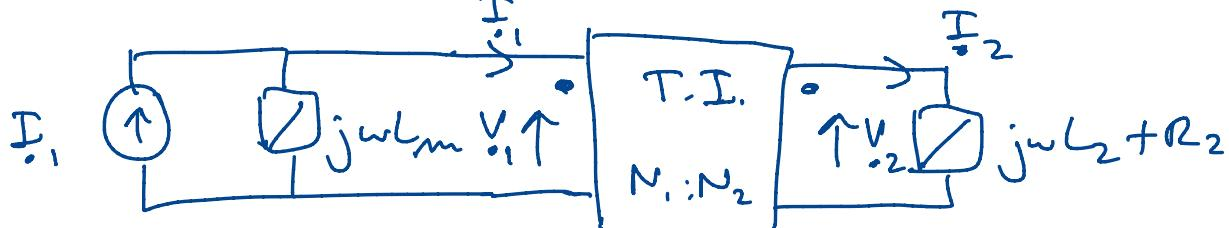
$$\tilde{\dot{I}}_1' = \dot{I}_1 - \frac{\dot{V}_1}{jwL_m} \quad \text{pero} \quad \frac{\dot{V}_2}{\dot{V}_1} = \frac{N_1}{N_2} \quad \text{e} \quad \frac{\tilde{\dot{I}}_1'}{\dot{I}_2} = \frac{N_2}{N_1}$$
