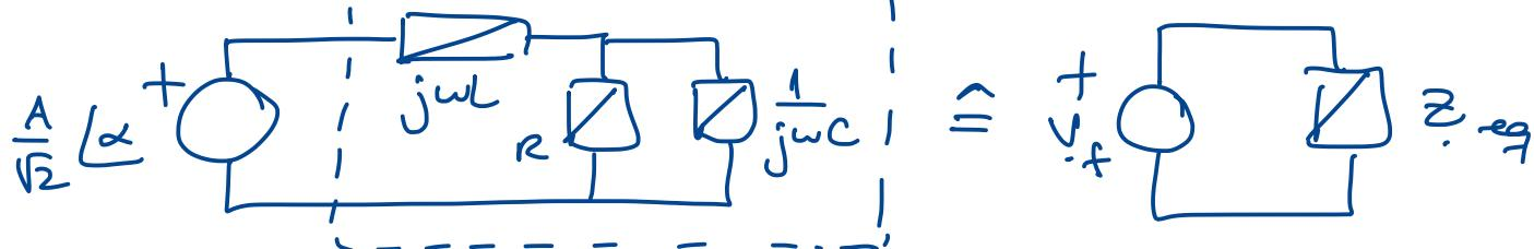
$$\begin{aligned} \text{en que } \bar{Z}_{eq} &= jwl + R \parallel \frac{1}{jwC} \\ &= jwl + \frac{R}{(1+jwRC)(1-jwRC)} (1-jwRC) \\ &= \frac{R}{1+(wRC)^2} + j \left[ wl - \frac{wR^2C}{1+(wRC)^2} \right] \end{aligned}$$
