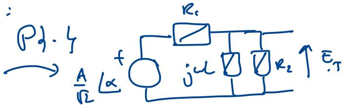
$$\begin{aligned} E_T &= \frac{j\omega L / R_2}{R_1 + j\omega L / R_2} \cdot \frac{A}{R_2} \angle \alpha \\ &= \frac{j\omega L R_2 \frac{A}{R_2} \angle \alpha}{R_1(j\omega L + R_2) + j\omega L R_2} \end{aligned}$$
