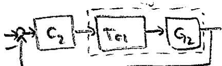
$$\text{Dónde } T_{01} = \frac{4(p_1 s + p_0)}{s^2 + 2\zeta w_m s + w_m^2} \quad \left\{ \begin{matrix} M=3 \\ r=1 \text{ (antigüedad)} \\ \Rightarrow M_C=3 \end{matrix} \right.$$
