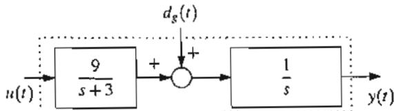
$$(a) G_o(s) = \frac{9}{s(s+3)} = \frac{B_o}{A_o} \quad C(s) = K_p + \frac{K_I}{s} = \frac{1}{3} + \frac{1}{9s} = \frac{3s+1}{9s} = \frac{P}{L}$$
