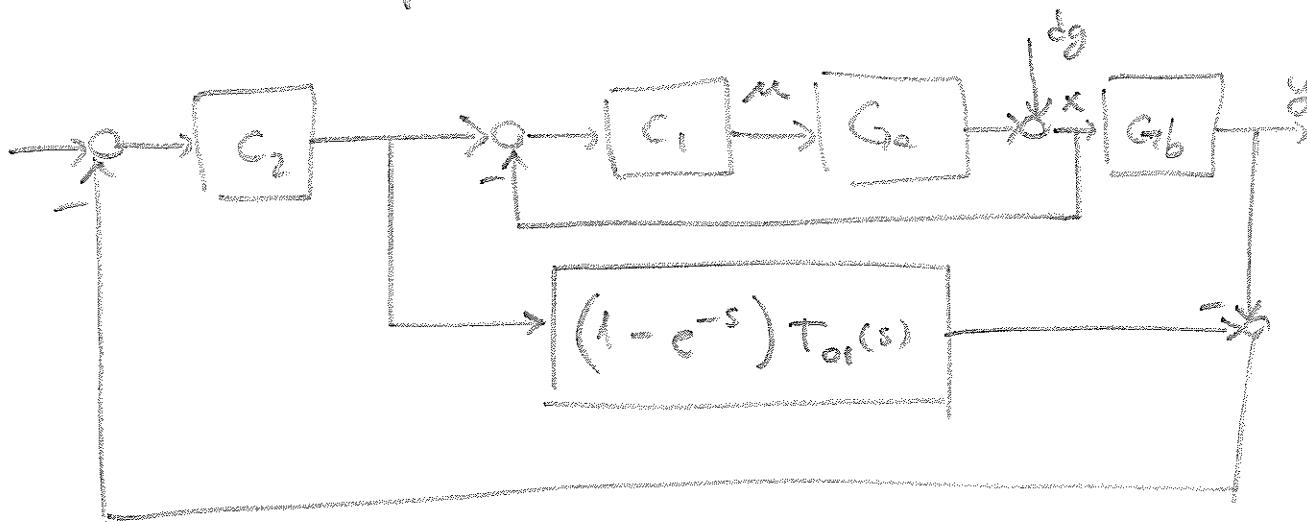
$$\text{en que } T_{01} = \frac{G_1 G_a}{1 + G_1 G_a} = \frac{B_0 P_1}{A_{01}} = \frac{B_0 z}{A_{02}} = \frac{(s+10)(P_2 + P_1)}{(s+5)(s+2) \underbrace{z}_{\text{asignar}}}.$$
