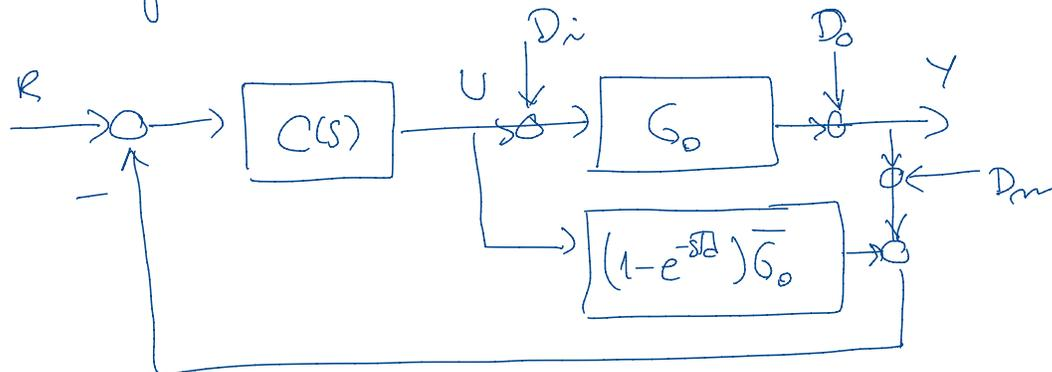
m que G\_o\_bar = K / (\tau s + 1)^2    G\_o = G\_o\_bar e^{-sT\_d}    C = (p\_2 s^2 + p\_1 s + p\_0) / (s(s + l\_0))
