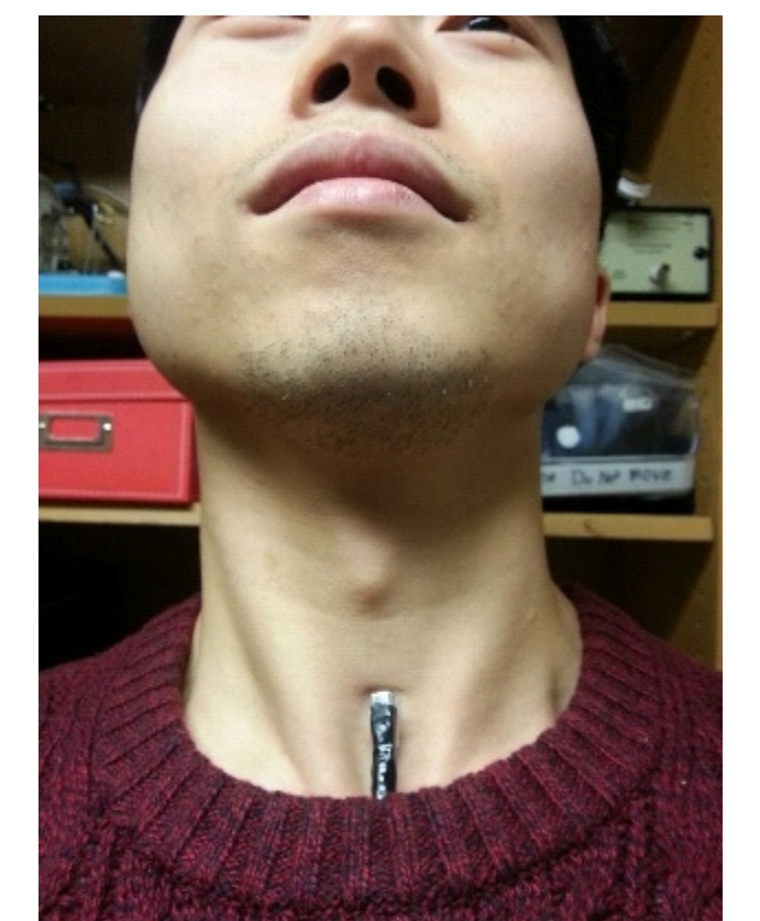
Fig 3. Example of accelerometer placement on the skin of the anterior neck.
