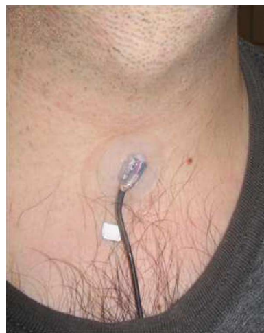
Fig. 5. (Color online) The accelerometer sensor mounted subglottally on the neck skin with double-sided tape.
