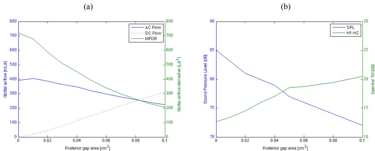
**FIGURE 3.** Effect of the posterior glottal gap on selected glottal measures. (a) Aerodynamic measures (b) Acoustic measures
